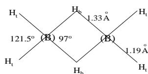
The distance between the two non-bonded boron atoms is 177 pm.
