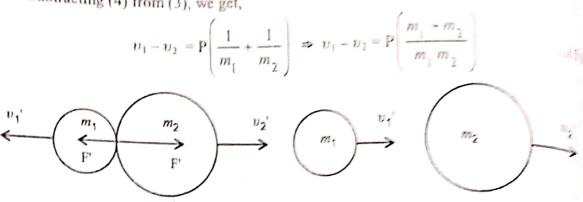
After the instant of maximum compression, the period of restitution begins and another system of forces comes into existence which helps the two spheres recover their original shape. These forces are also large and act for a very small period  $\tau'$ , say. Let  $v'_2$  be the velocities of the two spheres just after the impact.
