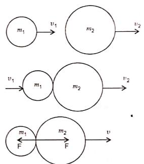
Let v be the common velocity of two spheres when the compression is maximum. Then, for the two spheres, we have,
