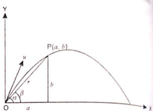
Art-10. Find the equation giving the two times corresponding to the two directions of projection for a projectile to hit a given point with a given velocity of projection. Show that product of times is
