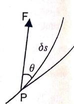
$$\therefore \frac{dW}{dt} = \underset{\delta t \to 0}{\text{Lt}} \frac{\delta W}{\delta t} = \underset{\delta t \to 0}{\text{Lt}} \frac{(F \delta s \cos \theta)}{\delta t}$$
