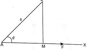
In the figure force F acts along AX, the displacement is AB = s making an angle  $\theta$  with AX and BM  $\perp$  AX so that
